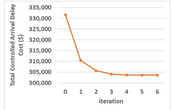
Figure 4 Total Controlled Arrival Delay Cost vs. iteration (2-opt-swap)
