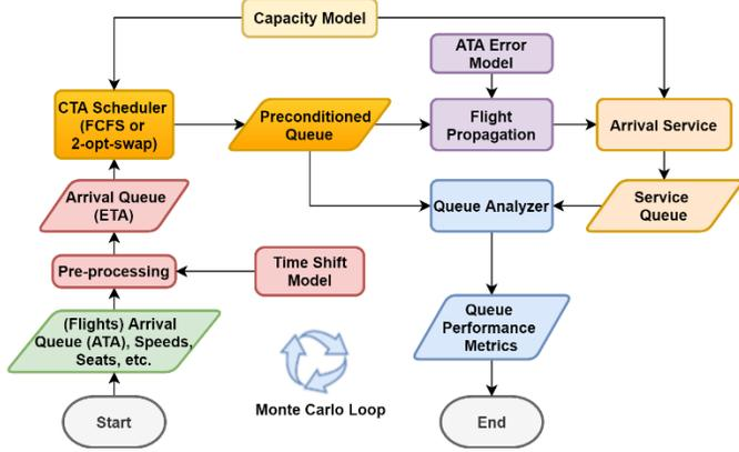
Figure 3. Simulation System Flow Chart
