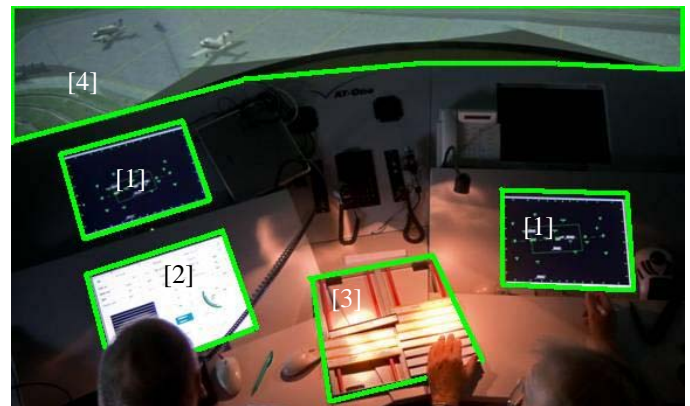
Figure 2. Design of working positions in the tower simulator compasses [1] RADAR, [2] weather display, [3] flight strips, [4] far view.
