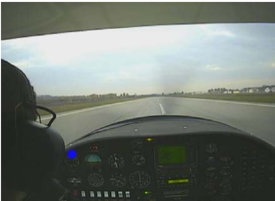
Figure 3: The blue dot represents the gaze fixation. Note that the pilot is focusing on the airspeed instrument to check the rotation speed (Vr), just before taking-off
