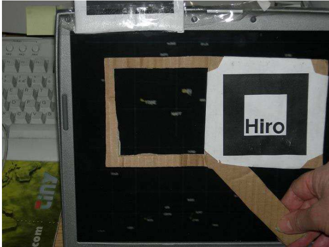
Figure 2. The tangible lens, implemented with the ARToolkit. The area inside the cardboard "lens" is a magnified view of that region of the airspace.
