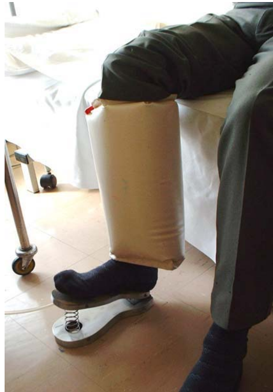
Figure 5. Volunteer with right leg resting on Test Jig A.
